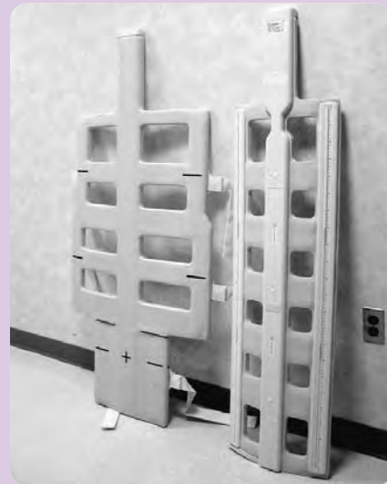
Figure 17 shows a 12-element peripheral vascular array coil designed for use during peripheral run-off MRA examinations. The coil is divided into anterior and posterior halves. The patient lays on the larger posterior half of the coil and the anterior half is placed on top the patient. The coil elements are activated in three groups during the imaging sequence: top, middle, and bottom stations. This coil is designed to provide coverage from the renal arteries to the feet.
