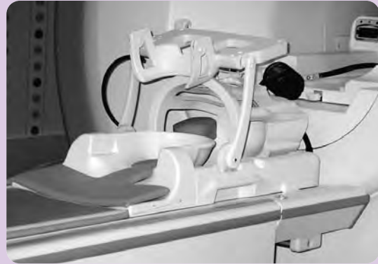
Figure 14. An example of a neurovascular array coil. The coil elements are arranged so the head can be imaged alone or in combination with the cervical spine, soft tissue of the neck, or carotid MRA imaging sequence. The head-only part of the coil can be activated while the neck portion remains inactive if imaging only the brain. When performing carotid MRA, the coverage requirements are from the aortic arch to the Circle of Willis; in this case both the head and neck portions of this coil can be activated together and receive signal in unison.
