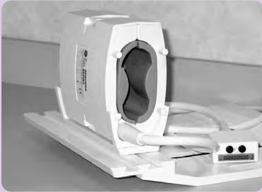
Figure 15. This 3-element array coil is designed specifically for imaging the wrist. The small coil element design ensures high SNR, enabling high resolution images.
