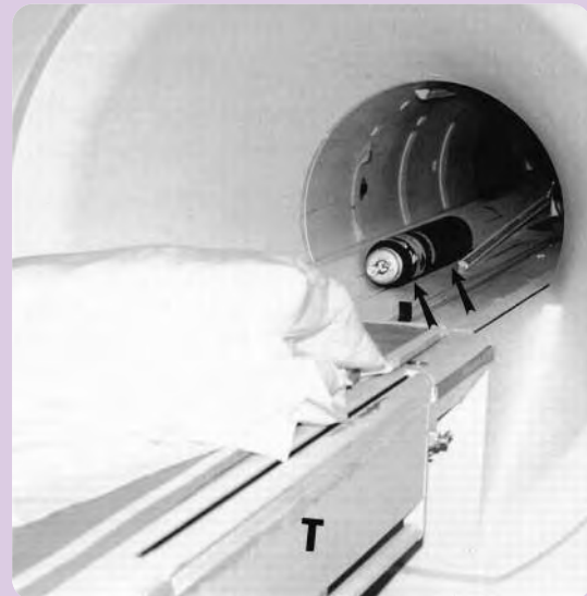
Figure 6. A portable ferromagnetic anesthesia tank that was pulled into the magnet. Although nobody was injured, the magnet sustained $50,000 of damage and a loss of one week's operating time. 4
