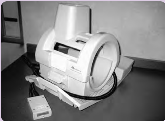
Figure 16. This quadrature design transmit-receive coil is used for knee and foot/ankle imaging. Note the column at the top for distal foot imaging and right-angle ankle positioning.
